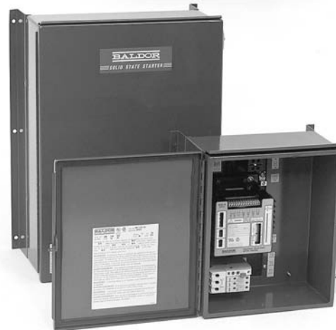
Figure 23b Solid-state soft starter rated 5 hp, 460 V, 60 Hz. Start-up time adjustable 5–50 s; initial torque adjustment 0–75%; current limit schedule 75%–400%; kick-start time adjustable 0–1.5 s. In background is 40 hp, 460 V soft starter. (Courtesy of Baldor Electric Company)
