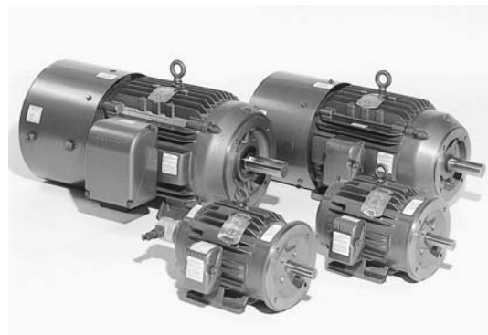
Figure 2 Two totally enclosed nonventilated (TENV) 2 hp, 1725 r/min cage motors are shown in foreground and two 30 hp, 1780 r/min totally enclosed blower-cooled motors (TEBC) in background. These 3-phase, 460 V motors are intended to operate at variable speeds ranging from a few revolutions per minute to about 3 times rated speed.
