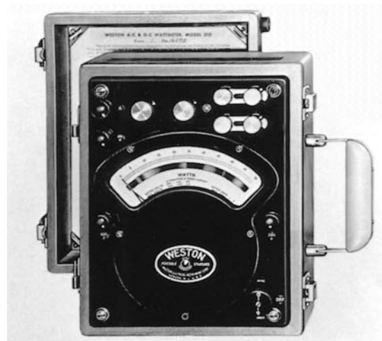
Figure 3 Example of a high-precision wattmeter rated 50 V, 100 V, 200 V; 1 A, 5 A. The scale ranges from 0-50 W to 0-1000 W. (Courtesy of Weston Instruments)
