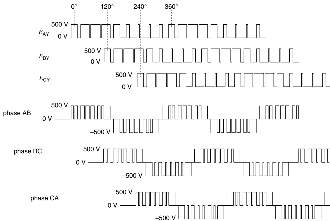
Figure 97 Three-phase PWM voltages produced by a dc-to-ac converter operating at a carrier frequency of 540 Hz with a 500 V dc input. Top: E_{AY} , E_{BY} , E_{CY} outputs, peak sinusoidal component = 200 V. Bottom: E_{AB} , E_{BC} , E_{CA} outputs, peak 60 Hz sinusoidal component = 346 V, RMS value = 245 V.
