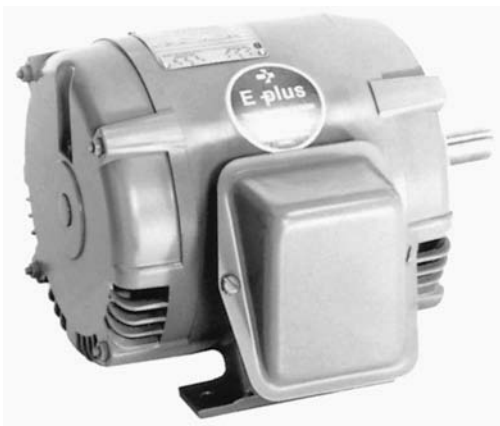
Figure 1 Energy-efficient, drip-proof, 3-phase, squirrel-cage induction motor rated 230 V/460 V, 3 hp, 1750 r/min, 60 Hz. (Courtesy of Gould)
