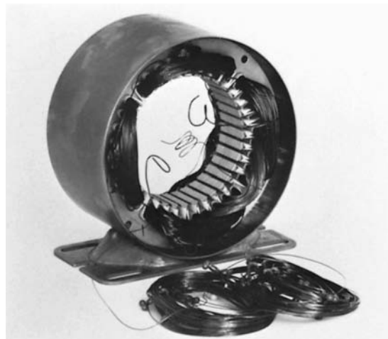
Figure 2c Four poles of the auxiliary winding straddle the main winding. (Courtesy of Lab-Volt)
