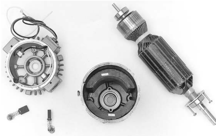
Figure 30 Permanent magnet motor rated 1.5 hp, 90 V, 2900 r/min, 14.5 A. Armature diameter: 73 mm; armature length: 115 mm; slots 20; commutator bars: 40; turns per coil: 5; conductor size: No. 17 AWG, lap winding. Armature resistance at 20°C: 0.34 Ω.
