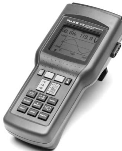
Figure 45 This portable instrument, the “Power Harmonics Analyzer” can measure the total harmonic distortion (THD) of a voltage or current up to the 31 st harmonic. It can also measure the active, reactive and apparent power in a 3-phase circuit, and its power factor. It also gives a readout of the K factor of a current. (Courtesy of Fluke Electronics Canada Inc.)
