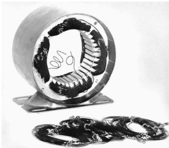
Figure 2b Four poles of the main winding are inserted in the slots.
