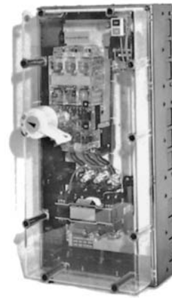
Figure 18 Three-phase, across-the-line combination starter, 150 hp, 575 V, 60 Hz. The protruding knob controls the disconnecting switch; the pushbutton station is set in the transparent polycarbonate cover. (Courtesy of Klockner-Moeller)
