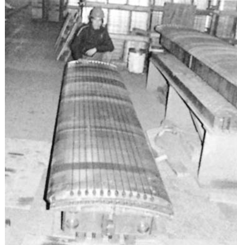
Figure 6 Salient-pole of a 250 MVA generator showing 12 slots to carry the squirrel-cage winding.
