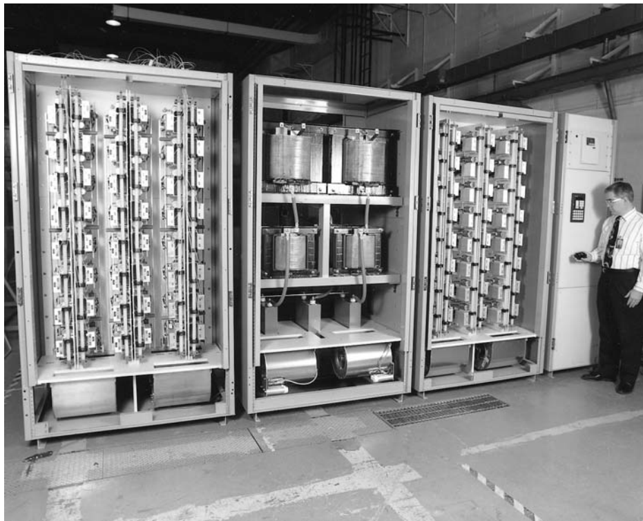
Figure 32 This \pm 2 MVA converter assembly can be used in either a shunt or series compensator (DSTATCON or DVR). (Courtesy of Westinghouse Electric Corporation)
