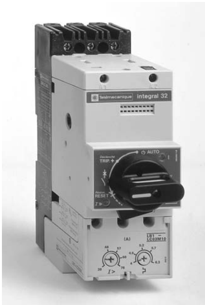
Figure 21 Special self-protected starter rated at 40 hp, 460 V, 60 Hz. In addition to a short-circuit capability of 42 kA at 460 V, it features adjustable thermal and magnetic trip settings. Overall dimensions: 243 mm high, 90 mm wide, 179 mm deep. (Courtesy of Telemecanique, Groupe Schneider)
