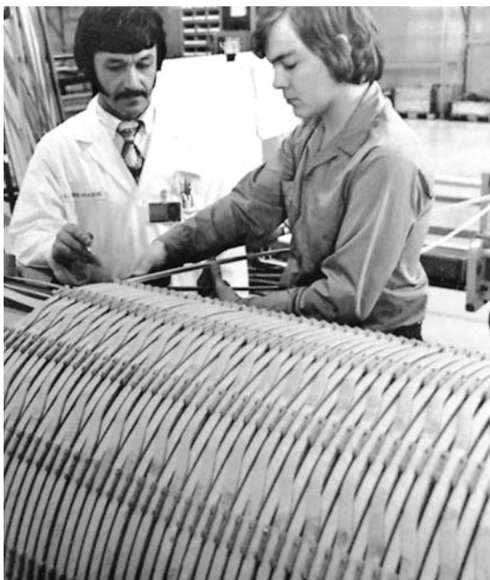
Figure 9c Primary winding of a large transformer; rating 128 kV, 290 A. (Courtesy ABB)
