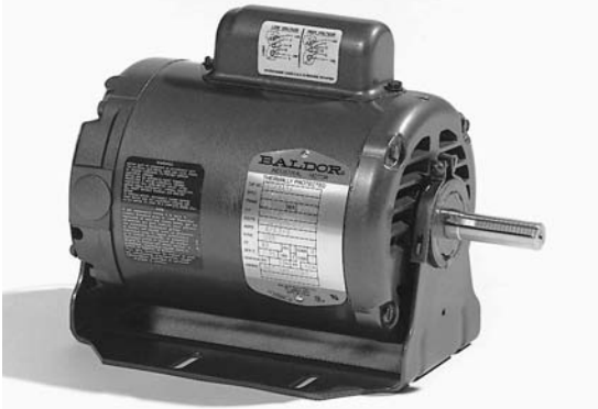
Figure 15 Single-phase capacitor-start motor supported in a resilient-mount cradle to reduce the vibration and noise transmitted to the mounting surface. Motor rated at 1/3 hp, 1725 r/min, 230 V, 60 Hz has a full-load current of 3.0 A, efficiency of 60 percent, and power factor of 60 percent. Other characteristics: no-load current: 2.6 A; locked-rotor current: 13 A; locked-rotor torque: 3.6 pu; breakdown torque: 3.0 pu; service factor: 1.35; total weight: 10 kg; overall length including shaft: 278 mm; overall height: 232 mm. (Courtesy of Baldor Electric Company)
