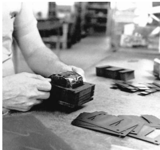
Figure 9b Stacking laminations inside a coil.
