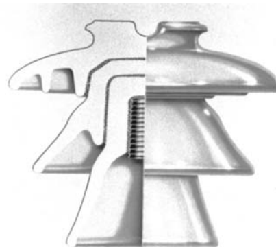
Figure 2 Sectional view of a 69 kV pin-type insulator. BIL: 270 kV; 60 Hz flash-over voltage under wet conditions: 125 kV. (Courtesy of Canadian Ohio Brass Co. Ltd.)
