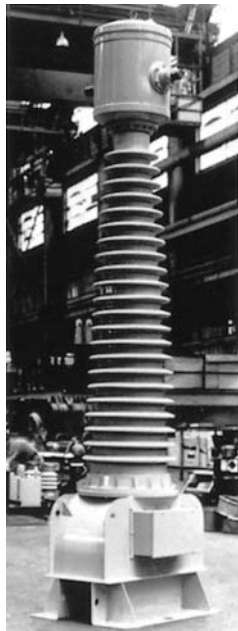
Figure 14 500 VA, 100 A/5 A, 60 Hz current transformer, insulated for a 230 kV line and having an accuracy of 0.6%. (Courtesy of Westinghouse)
