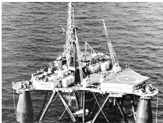
Figure 25 This floating oil derrick provides its own energy needs. Four diesel-driven generators rated 1200 kVA, 440 V, 900 r/min, 60 Hz supply all the electrical energy. Although ac power is generated and distributed, all the motors on board are thyristor-controlled dc motors. (Courtesy of Siemens)
