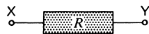
Figure 11 Current may flow from X to Y or from Y to X.
